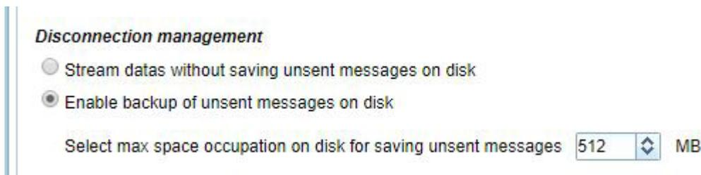
Figure 66. MQTT service: Disconnection management settings
