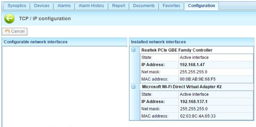
Figure 3. Network card data and setup of Ethernet and Wi-Fi
